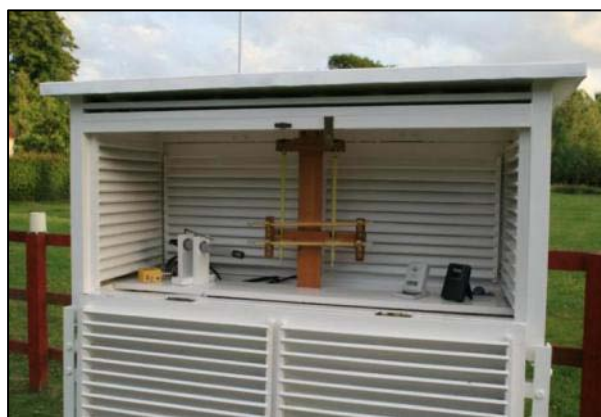
Figure 4 – Conventional Stevenson screen layout, showing maximum and minimum sheathed liquid-in-glass thermometers (mounted horizontally) together with the Vaisala HMP45C temperature and humidity sensor used in this comparison (grey cylinder, left of screen). This photograph was taken on 14 June 2009.
